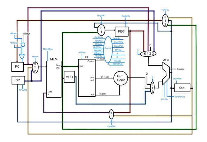
Each instruction cycle begins with the fetch at PC, from there the processor is able to complete all operations. All control bits and paths are as labeled above, and support a full range of basic processor operations.
